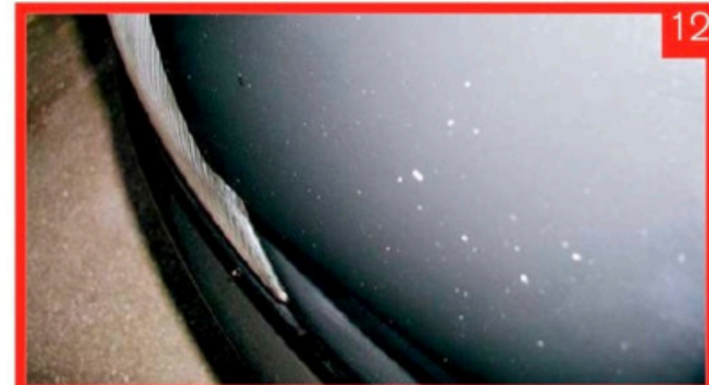
Large area of chipping requiring boot lid to be re-painted
