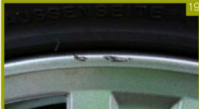
Scuffs up to 25mm on alloy wheels are acceptable
