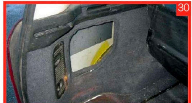
Torn covering and trim in boot area
