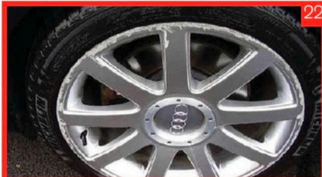
Wheel damage due to kerbing
