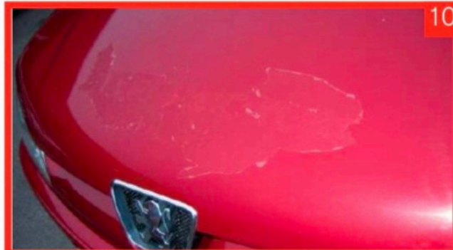
Adhesive residue following removal of company badges and logos
