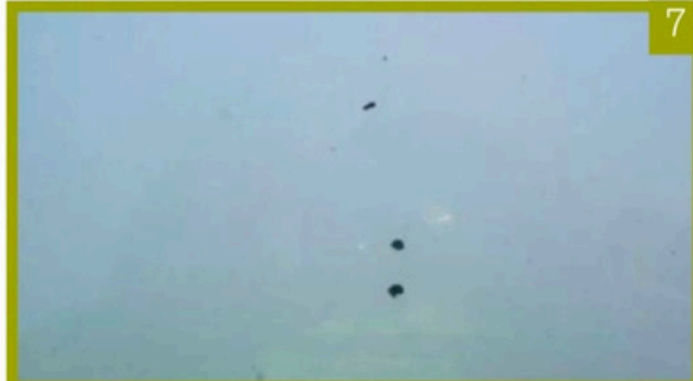
Small areas of chipping are acceptable if there is no corrosion present
