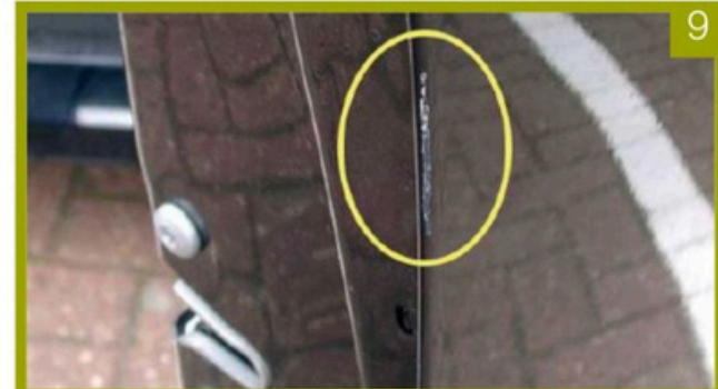
Small areas of chipping on door edges are acceptable
