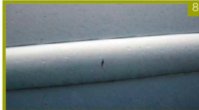
Scratches up to 25mm are acceptable except where primer or bare metal is showing
